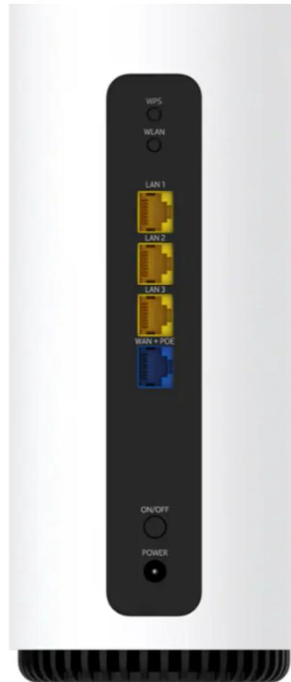
Plug in the power of the Nokia router into a reliable 120VAC power supply. The internet service modem will be connected by your Dash Internet installer.
